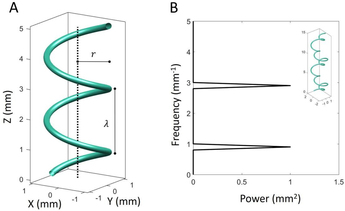
Figure 1: Helical transform. (A) An helix is a function  $f$  defined as  $(x(t) = r \sin(2\pi kt), y(t) = r \cos(2\pi kt), z(t) = k\lambda t)$ , where  $r$  is the radius of the helix,  $k$  is its frequency, and  $\lambda$  its wavelength. (B) The helix transform decomposes a root trajectory into the contribution of various helical frequencies that compose it. In this example, a root trajectory is composed of two frequency  $f(t) = \psi_1(t) + \psi_3(t)$
